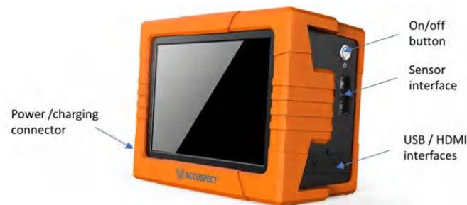
Figure 9. Self-designed and constructed EC testing instrument.
