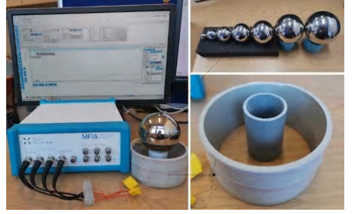
Fig. 4 Experimental setup and measured stainless-steel spherical shells
