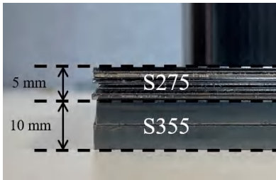
Fig. 13. Test pieces of stacked S355 and S275 mild steel plates
